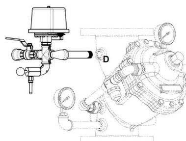
\*If a pressure switch (Pos. 7) with an outer thread is used, the Hex. nipple located underneath (Pos. 4) is not required.
