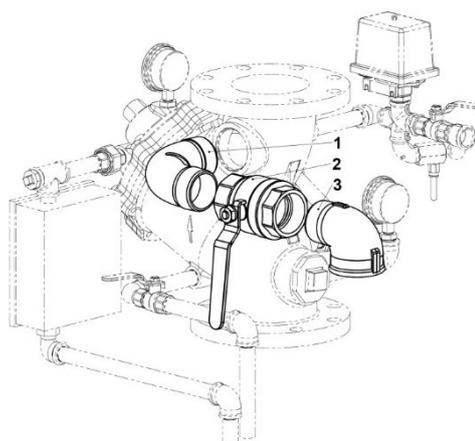
**6.8 Inspection and drain connection**
